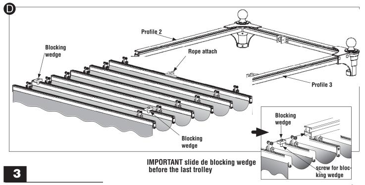
Slide the trolleys one by one in the profiles 2 and 3.
