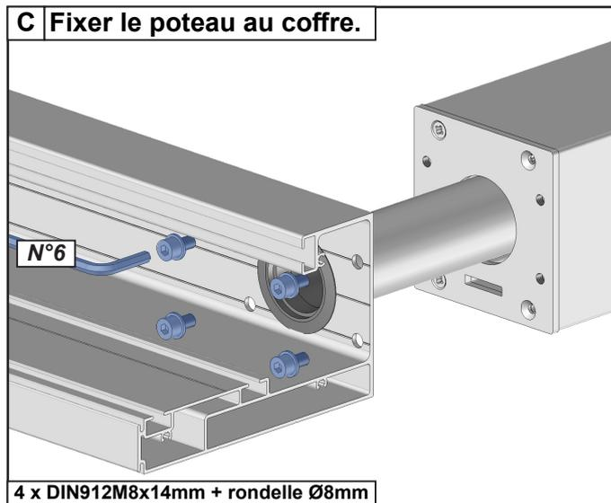
4 x DIN912M8x14mm + rondelle Ø8mm
