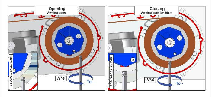
Limit switch: Turn the screw towards the '+' for more closing or opening, towards the '-' for less closing or opening. Carry out a test to validate the stop. Warning: the motor will go into thermal protection after 2 successive lifts and 1 successive lowering.
